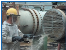
Removal of a hardened polymer from heat exchanger tubes using manually operated waterjetting tools.
