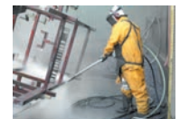
Removing bonded paint from automotive assembly line carrier.
