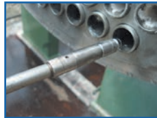
Removal of a hardened polymer from heat exchanger tubes using manually operated waterjetting tools.
